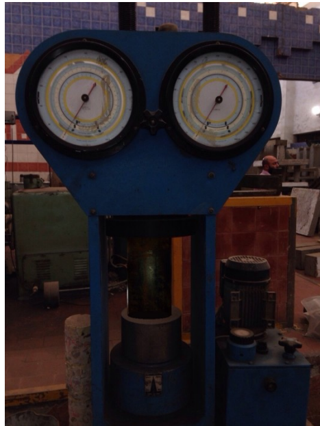
Figure 1: Compression test setup of the confined concrete cylinders.
